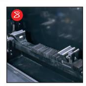
Bed Bar Mounting System allows the bed bar assembly to remain straight and stable throughout the grinding process without inducing stress.
