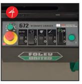
**Electronic Control Panel** contains independent switches for all grinder functions and meets all safety requirements including an emergency stop button. Magnet-ON indicator light is included.
