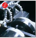
Flood Coolant controls dust, allows fast grinding time by controlling the bedknife temperature during the grind, and aids in producing a high quality surface finish.
