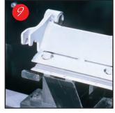
Alignment Gauge simplifies and virtually eliminates set-up time. The forward and upright position is used for alignment of the bedknife. After alignment, the gauge is stored in an out-of-theway position.
