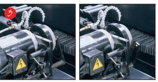
Diamond Wheel Dresser allows the operator to redress the grinding wheel. The permanently attached dresser stores easily out of the way during grinding and requires minimal adjustment for dressing.
