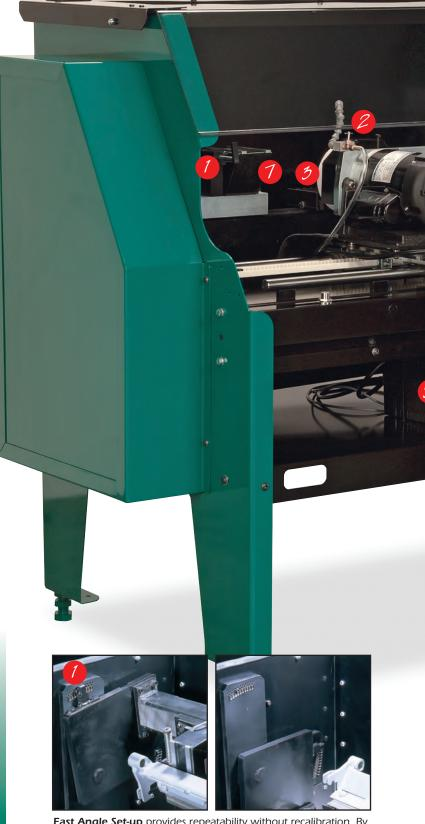
**Fast Angle Set-up** provides repeatability without recalibration. By setting the Angle Stops once, the 672 can grind the same angles over and over. This is the market's fastest method of setting the desired angle.
