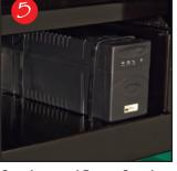
Supplemental Power Supply Supplemental Power Supply protects the operator in the event of electrical supply interruption holding the bedbar in place. It is easily accessible in a storage area, which can hold tools or other bedknives that need to be ground.
