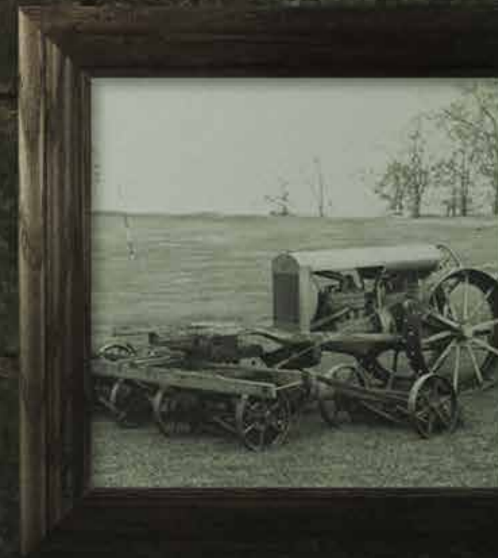
The famous Minikahda Mower from 1921. Mounting five lawn mowers onto the front of a farm tractor, Toro® initialized the motorized golf course equipment industry.
