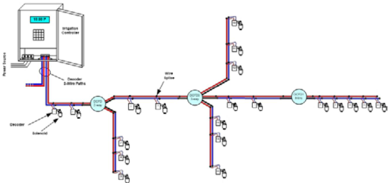
Note that the Decoder Cable Fuse Devices have been strategically installed at the points where cables split in different direction. Or it can be installed in long straight wire sections to isolate it in half. These are the obvious location where one would undo the splices when troubleshooting and trying to isolate the section of the system that is causing the fault.
