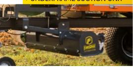
This optional extra fitted to Foresteel trailers' frame and connected directly to vacuum makes collecting leaves and debris possible with any towing vehicle. The unit is towed under the trailer's frame, it is height adjustable and copies land on two rollers. It's copying capabilities make going over smaller bumps and hills easy and intuitive.
