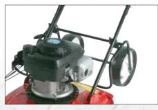
HI-RISE KIT 02619: eHoverPro 450 and HoverPro 450 only Simply bolt to existing deck to increase height of cut by 35 mm.
